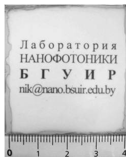
Fig. 3. Photograph of PAA membrane 4 \times 4 cm in size and about 100 \mu\text{m} thick. In order to reveal its high transparency, the membrane was put onto a sheet of a white paper with the printed name of laboratory in Russian and the author's email address.
